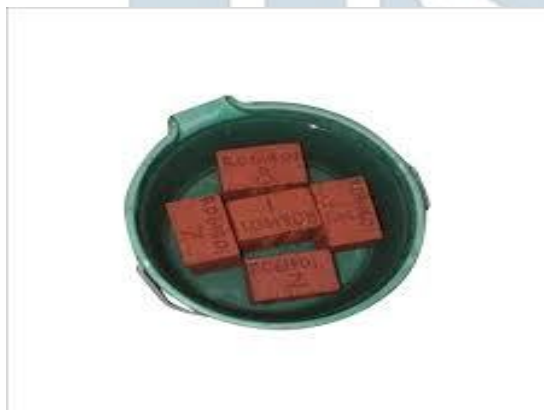
Figure 8: Bricks Water Absorption Test
