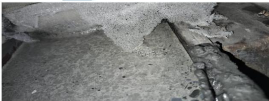
Figure 3: Emckcrete 90DS mixing with 6mm Down concrete design mix
