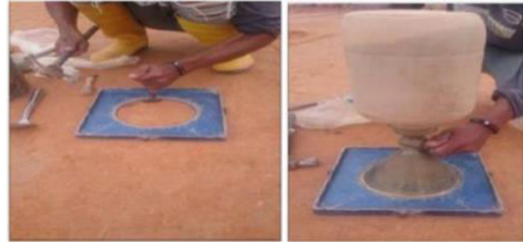
Figure 4: Field testing of sand cones
