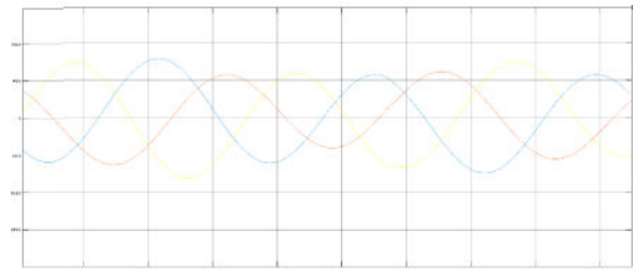
Figure 27: Voltage Output from the inverter with modified voltage optimizer active power controller
